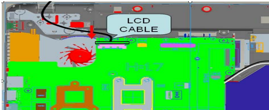
Figure 4-8-9 Connecting LCD harness to the mother board
